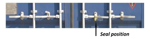
When locking the door, lock door cam must be closed completely.
